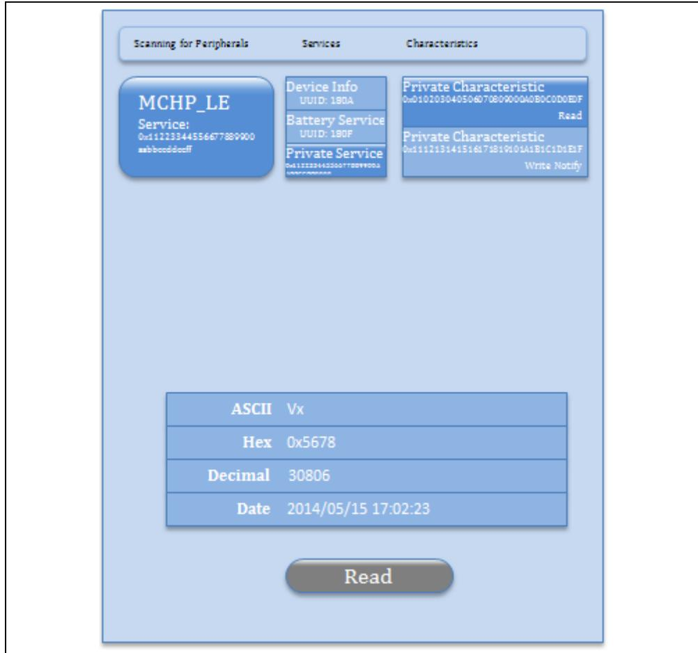
The BTLE BROWSER APP can also write or start notification on characteristic 0x111213141516171819101A1B1C1D1E1F. The effect is the same as operating on a public characteristic. The only difference to the RN4020 module is that the public characteristic has a short 16-bit UUID, while the private characteristic has a long 16-byte UUID.
