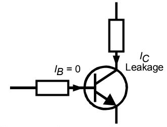
Leakase current Ic=0.170mA Older Germanium types however can suffer from significant collector leakage current, particular at high temperatures (leakage current can be <u>very</u> temperature dependant).
