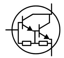
The *Atlas DCA* can detect the resistor shunt if it has a resistance of typically less than  $60k\Omega$ .
