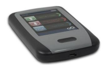
The EL-DataPad allows users of Lascar's EL-USB data loggers to configure their units and download data and view logging results on-the-spot rather than removing the logger from the environment being measured and taking it to their PC. This allows continual logging with shorter breaks in data collection, less travel for the user, on-site data collection in graph, legend and summary format and the ability for users to reconfigure loggers in 'the field'.
