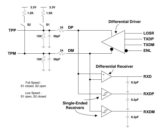
The following figure describes the key parameters of the differential driver – values for these parameters for high and low speed operation are listed in the tables overleaf. The above figure includes details of the loading for this testing.
