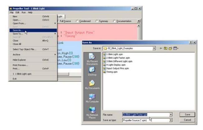
The Timing object's Pause method has a duration parameter — a value that says how long to pause for. All you have to do to make the light blink faster is pass a smaller value to this duration parameter. Let's try 100.
