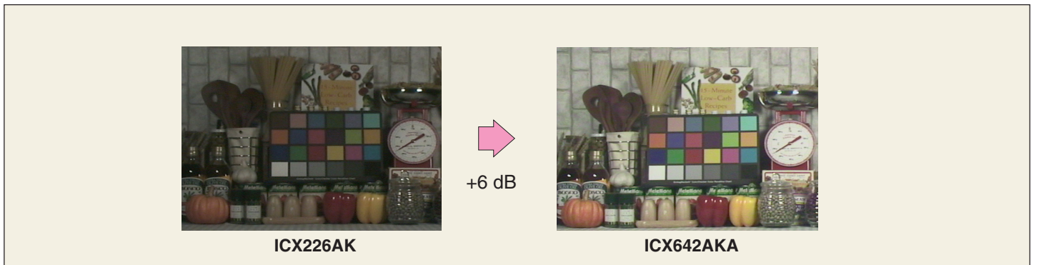
■ Photograph 1 Sensitivity Characteristics Comparison (Using the Sony CXD3172AR)
