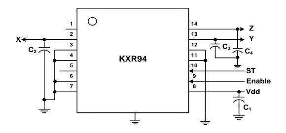
3. When not connecting the self test pin to a digital I/O port of a microcontroller, Kionix recommends connecting the self test pin to ground.
