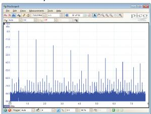
With the click of a button, you can open a new window to display a spectrum plot of selected channels up to the full bandwidth of the oscilloscope. A comprehensive range of settings gives you control over the number of spectrum bands, window types and display modes.
