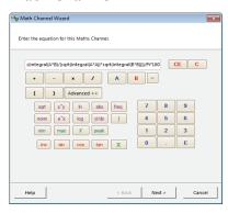
With PicoScope 6 you can perform a variety of mathematical calculations on your input signals and reference waveforms.
