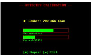
Press the appropriate button to repeat the test, or to exit.
