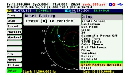
The internal disk drive can be optionally formatted. Press the Select [•] button to format the disk or any other button if only a reset to factory defaults is required.
