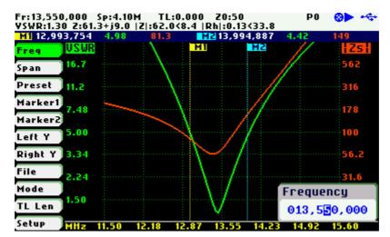
(ii) Use Navigator A to highlight «Freq» in the main menu on the left side of the display. Then use Navigator B to change the frequency. The frequency will change according to the current frequency multiplier. The frequency multiplier can be changed from the popup dialog, see (i) above.
