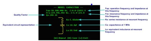
The internal procedure performed by the analyzer is as follows: the analyzer measures the impedance at 1 MHz and at the desired operating frequency. Then it searches for the self-resonant frequency and measures the impedance at this point. The following parameters are extracted from these measurements:
