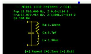
The figure below describes the measured parameters:
