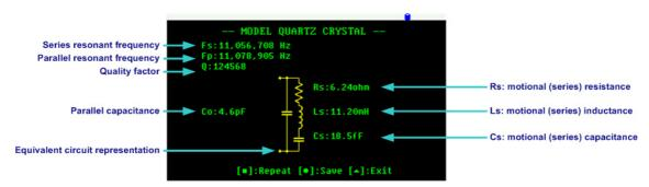
The process starts by searching for the series and parallel resonant frequencies. The start scan frequency is taken from the specified frequency value. The scan range is +1 MHz up and -1 MHz down from this value.
