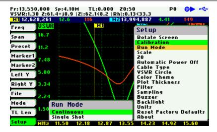
In continuous mode the analyzer is constantly sweeping provided that it is not in paused state. In single-shot mode the sweep automatically stops on completion. Press the Run/Hold [>||] button to start a new sweep. Notice that in the stop condition the power consumption is reduced, so using single-shot mode helps to increase the battery autonomy.
