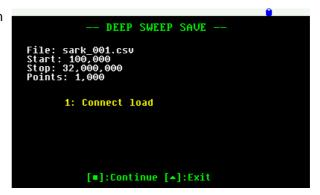
After completing the sweep scan, the analyzer will save the results of the sweep scan to the file.
