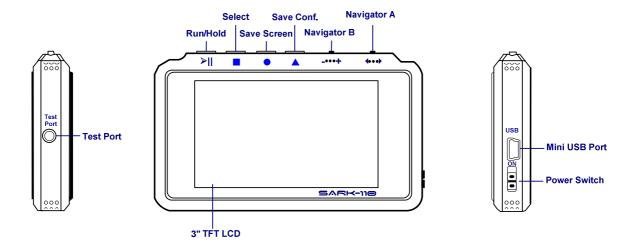
The unit has a Test Port located on its left side, to connect to the device under test. This receptacle accepts straight MCX plug connector types. The product pack includes an MCX to SMA female connector adapter and a 20-cm SMA plug to SMA female cable adapter.
