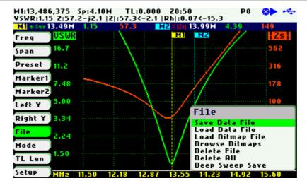
After selecting the "Save File" submenu option, enter the file name. By default, the file name has the format "sark\_xxx.csv" (or "sark\_xxx.tdr" for Cable Test mode), where xxx is an automatically assigned number. To change the file name, use Navigator B to change the character value and Navigator A to change the character position highlighted in inverse video. Press the Select [ ] button to validate the selection. Press any other button to cancel the operation.
