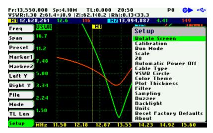
Use Navigator B to highlight the desired submenu setup option. Press the Select [■] button to validate the selection. Press any other button to cancel the operation.
