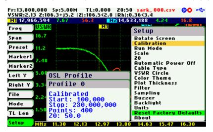
Once the calibration profile has been selected, choose **«Setup»** *«Calibration»* **«OSL** Calibration» to start the OSL calibration procedure.
