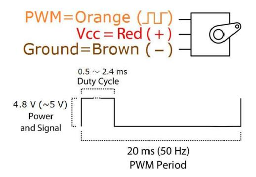
Position "0" (1.45 ms pulse) is middle, "90" ( $\sim$ 2.4 ms pulse) is all the way to the right, "-90" ( $\sim$  0.5 ms pulse) is all the way left.
