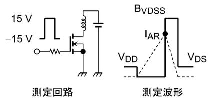
$$R_G = 25 \Omega, V_{DD} = 50 V \quad E_{AS} = \frac{1}{2} \cdot L \cdot I_{AR}^2 \cdot \left( \frac{B_{VDSS}}{B_{VDSS} - V_{DD}} \right)$$
