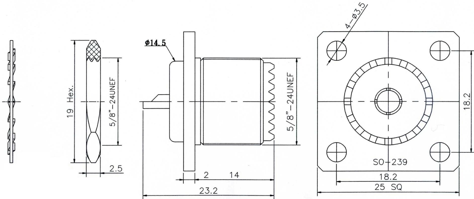
Dimensions Are In Millimeters
