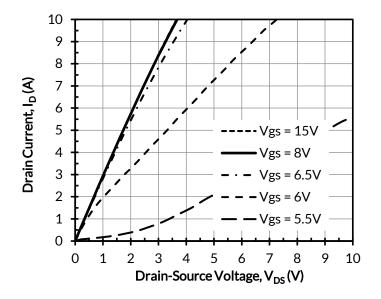
9 8 Drain Current, I<sub>D</sub> (A) 7 6 5 Vgs = 15V 4 Vgs = 8V 3 - Vgs = 6V 2 - Vgs = 5.5V 1 Vgs = 5V 0 0 2 3 5 10 1 Drain-Source Voltage, V<sub>DS</sub> (V)
