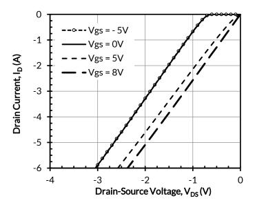
Figure 10. 3rd quadrant characteristics at T<sub>J</sub> = 25°C
