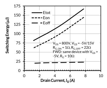
Figure 18. Clamped inductive switching energy vs. drain current at  $T_J = 25$ °C
