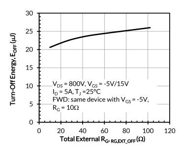
Figure 20. Clamped inductive switching turn-off energy vs.  $R_{G,EXT\ OFF}$
