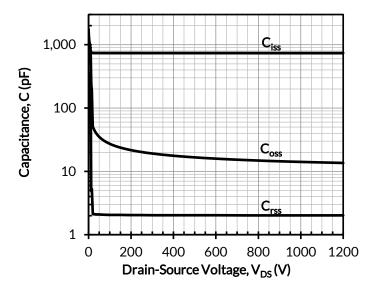
Figure 13. Typical capacitances at f = 100kHz and  $V_{GS} = 0V$
