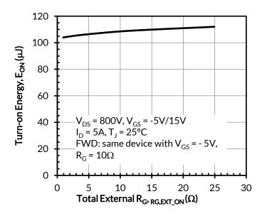
Figure 19. Clamped inductive switching turn-on energy vs.  $R_{\text{G,EXT\_ON}}$
