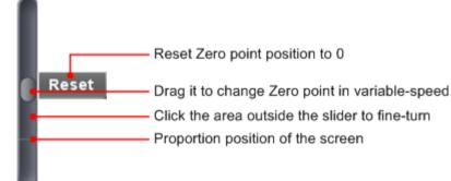
Drag the slider up to increase, down to decrease; the further from the center, the higher the changing speed is.
