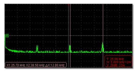
**Vamp Measurement:** Tick on "Amplitude", enter Home page->Math->FFT, then two light red lines represent Cursor 1 and Cursor 2 show along the horizontal direction on FFT window.
