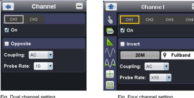
Fig. Dual channel setting To turn on/off channels
