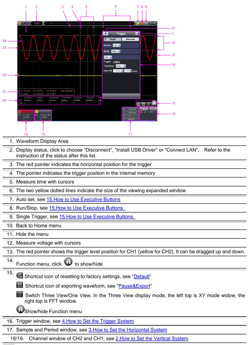
20. Display the measured type and value of the corresponding channel, see <u>6.How to Measure Automatically</u>
