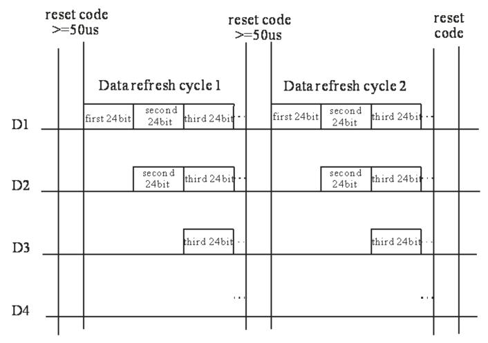
Note: The data of D1 is send by MCU, and D2, D3, D4 through IC internal reshaping amplification to transmit.
