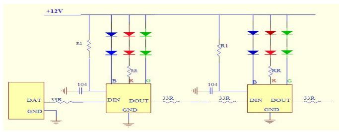
Note: WS2850 LEDs are recommended to ensure the light emitting consistence.
