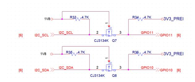
MILKV-Duo has not added external pull-up resistors to the pins with IIC functionality in consideration of interface function reuse. When other pins need to be multiplexed as IIC interfaces, external pull-up resistors need to be added and pulled up to 3.3V.
