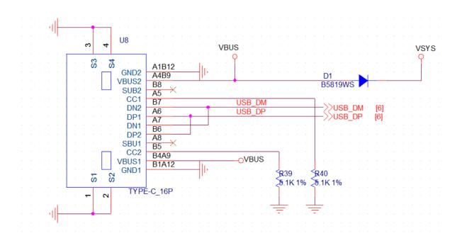
The MILKV-DUO can operate in USB Device mode for firmware burning and downloading when USB\_VBUS\_DET (PIN45/ADC2) is detected through a resistor-divided 5V\_USB\_IN and powered high. However, if the USB port is not being used for burning, USB\_VBUS\_DET (PIN45/ADC2) can be directly connected to ground, and the MILKV-DUO will operate in Host mode, enabling it to connect to external USB devices such as USB HUBs or USB 2.0 devices.
