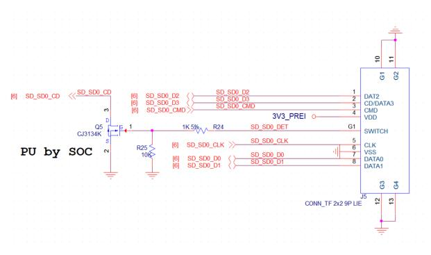
MILKV-DUO connects the SDIO0 interface to the TF card slot, allowing users to store system files in the TF card and boot the system from it. In addition, for the convenience of commercial customization users, SDIO0 is designed to be compatible with an SD NAND (default not mounted)
