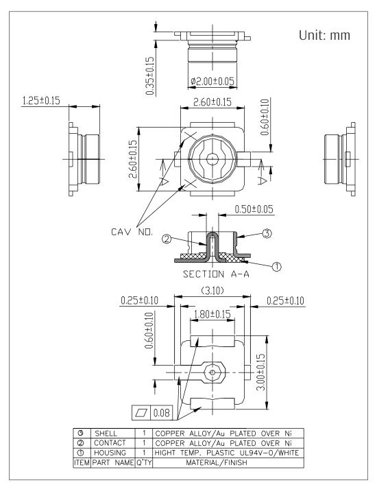
Figure 8: ESP32-WROOM-32U U.FL Dimensions
