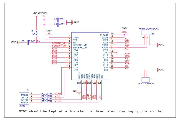
Figure 5: ESP32-WROOM-32D/ESP32-WROOM-32U Peripheral Schematics
