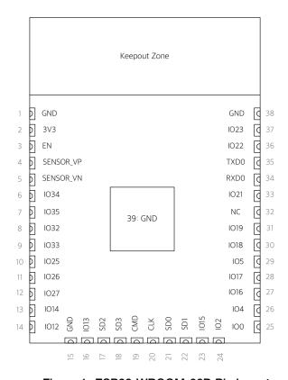
Figure 1: ESP32-WROOM-32D Pin layout
