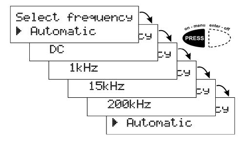
**Automatic** – The **LCR45** will attempt to use the most appropriate test frequency to suit the component being tested. This is generally the best option for most requirements. It will automatically and dynamically select between DC, 1kHz, 15kHz and 200kHz.
