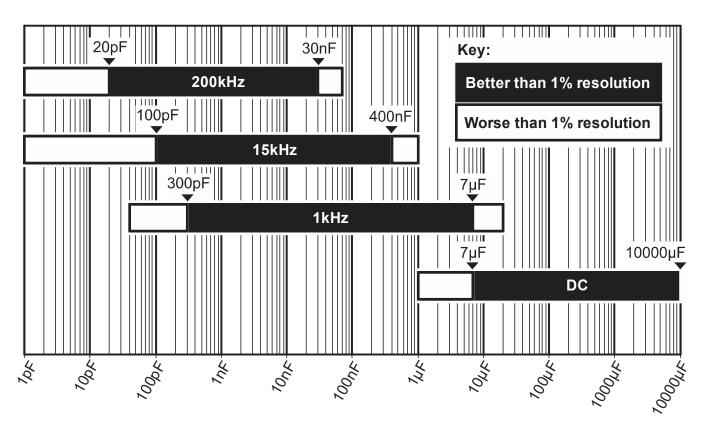
Measuring capacitance outside of the black bands will result in degraded measurement resolution (possibly worse than 1% of the measured value).
