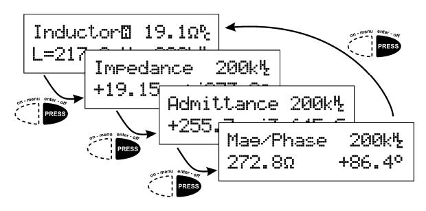
If the test frequency is set to DC (either automatically or manually) then it is not possible to show Impedance, Admittance or Mag/Phase. In those situations, you will see the letters N.  $\overline{A}$  displayed.
