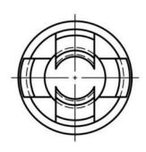
MOUNTING HOLE: Ø5 CHASSIS THICKNESS: 1.0~1.1
