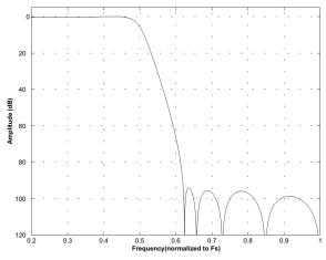
Figure 39. Quad-Speed (fast) Stopband Rejection
