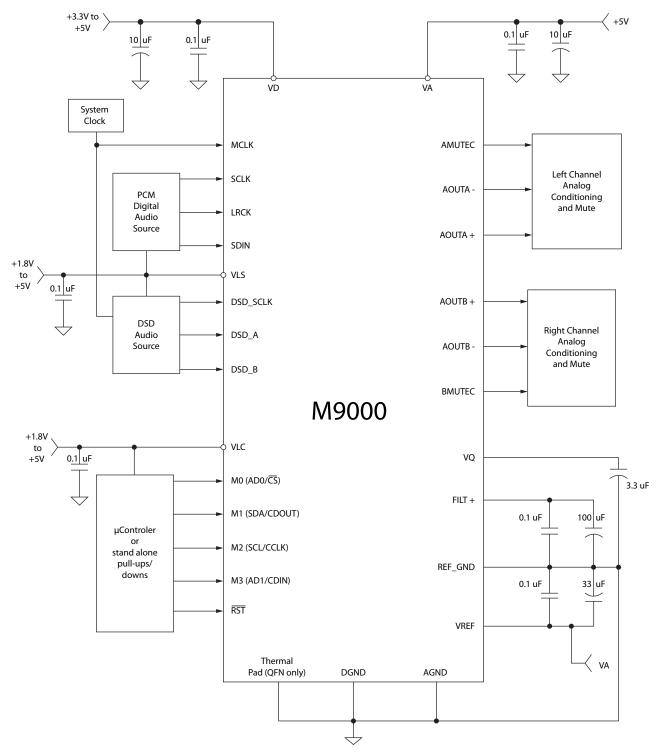
Figure 12. Typical Connection Diagram
