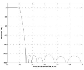
Figure 23. Single-Speed (fast) Stopband Rejection
