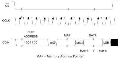
Figure 17. Control Port Timing, SPI Format (Write)
