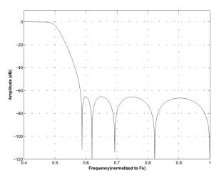
Figure 27. Single-Speed (slow) Stopband Rejection
