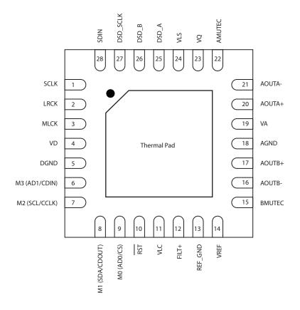
Figure 3. M9000 Pinout Drawing-QFN
