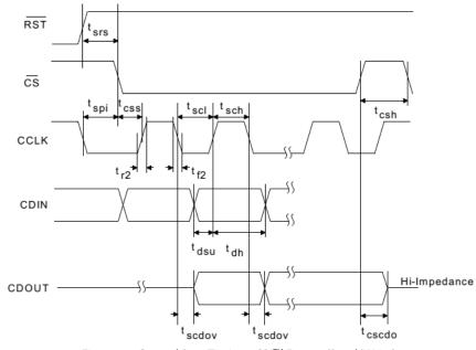
Figure 11. Control Port Timing - SPI<sup>™</sup> Format(Read/Write)
