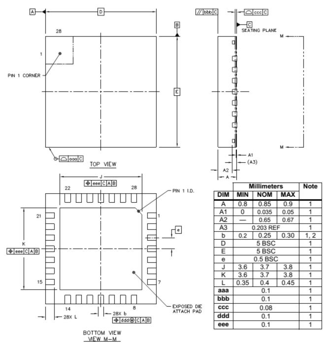
JEDEC #: MO-153 Controlling Dimension is Millimeters. Figure 22. 28L QFN Package Drawing
