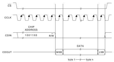
Figure 18. Control Port Timing, SPI Format (Read)
