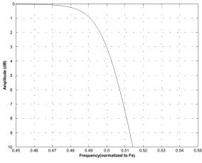
Figure 33. Double-Speed (fast) Transition Band (detail)
