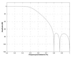
Figure 35. Double-Speed (slow) Stopband Rejection
