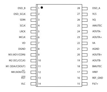
Figure 2. M9000 Pinout Drawing-TSSOP
