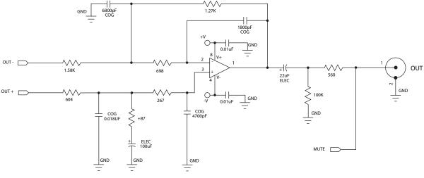
Figure 13. Recommended Output Filter
