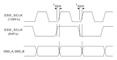
Figure 9. Direct Stream Digital - Serial Audio Input Timing for Phase Modulation Mode
