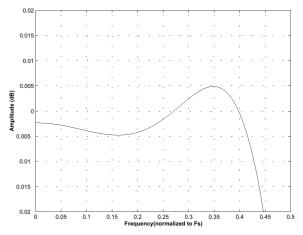
Figure 34. Double-Speed (fast) Passband Ripple
