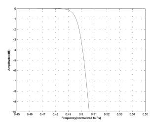
Figure 25. Single-Speed (fast) Transition Band (detail)
