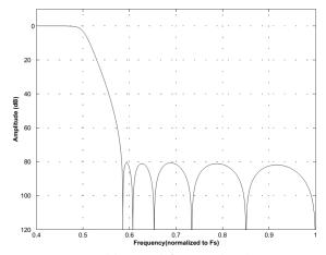
Figure 31. Double-Speed (fast) Stopband Rejection
