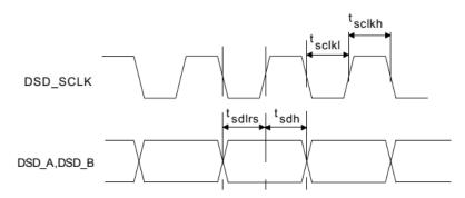
Figure 8. Direct Stream Digital - Serial Audio Input Timing
