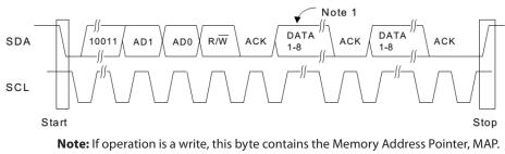
Figure 16. Control Port Timing, I<sup>2</sup>C Format
