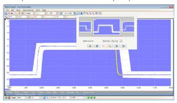
Connect the system under test, and PicoScope will highlight any parts of the waveform that fall outside the mask area. The highlighted details persist on the display, allowing the scope to catch intermittent glitches while you work on something else. The measurements window counts the number of failures, and can display other measurements and statistics at the same time. You can import and export masks as files.
