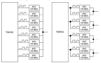
In parallel mode, multiple ADCs are sampled in phase on each channel increasing the resolution to 14 bits (see diagram) at 125 MS/s per channel (70 dB SFDR). If only two channels are required then resolution can be increased to 15 bits, and in single-channel mode all the ADCs are combined to give a 16-bit mode at 62.5 MS/s.
