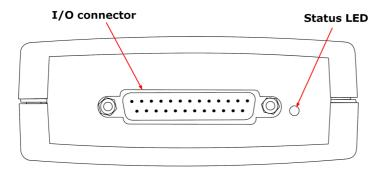
I/O connector: for the pin-numbering of the I/O connector, see I/O connector pins 1. The Pico PP545 Small Terminal Board is specially designed to connect to this socket to allow you to make connections to individual wires easily without soldering. If you need to use a ribbon cable to connect your signals to this socket, use the shortest possible length to avoid introducing too much crosstalk between the signals.
