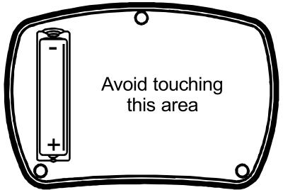
We recommend that the battery is replaced with a high quality battery equivalent to an **Alkaline AAA**, LR03 or MN2400 (1.5V). Replacement Alkaline AAA batteries are available from many retail outlets.
