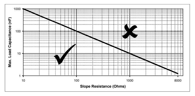
**Resistive Loading -** Depending on the selected test current range, the following resistive loads will influence Vz measurements by 1% or more:
