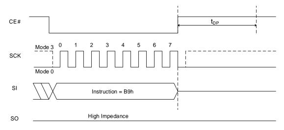
Figure 8.37 Enter Deep Power Down Mode Sequence In QPI Mode
