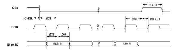
Figure 9.3 SERIAL INPUT TIMING (DTR Mode)
