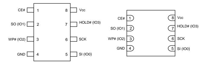
8-pin SOIC 208mil (Package: B) 8-pin SOIC 150mil (Package: N) 8-pin TSSOP (Package: D) 8-pin VVSOP 150mil (Package: V) 8-pin USON 2x3mm (Package: Y) 8-pin WSON 6x5mm (Package: K)
