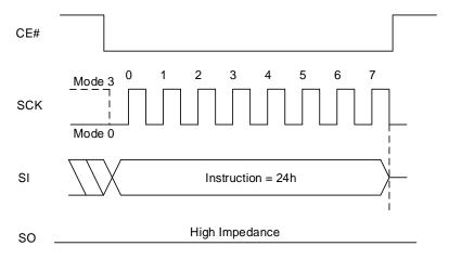
Figure 8.58 Sector Lock QPI Sequence In QPI Mode
