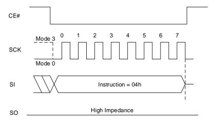
Figure 8.25 Write Disable Sequence In QPI Mode
