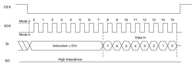
Figure 8.29 Write Status Register Sequence In QPI Mode
