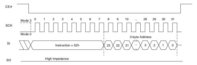
Figure 8.19 Block Erase (32KB) Sequence In QPI Mode
