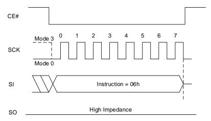
Figure 8.23 Write Enable Sequence In QPI Mode
