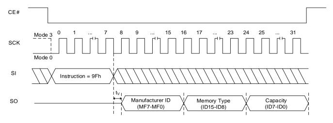
Figure 8.45 RDJDID and RDJDIDQ DJDIDQ (Read JEDEC ID In QPI Mode) Sequence
