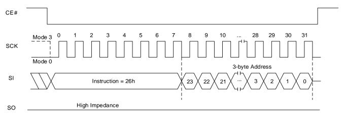
Figure 8.56 Sector Unlock QPI Sequence In QPI Mode
