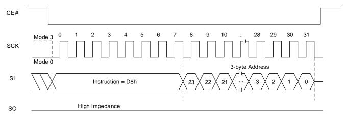
Figure 8.17 Block Erase (64KB) Sequence In QPI Mode
