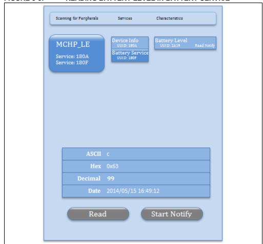
FIGURE 3-3: READING BATTERY LEVEL IN BATTERY SERVICE
