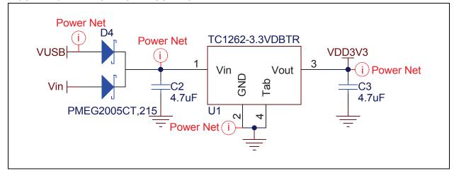
FIGURE A-7: DECOUPLING CAPACITOR FOR THE PIC18LF25K50-I/ML DEVICE
