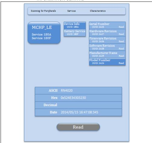
6. Read UUID "180F" to show one characteristic Battery Level with UUID "2A19". Reading the "2A19" characteristic shows this characteristic's property: readable and notification can be started.
