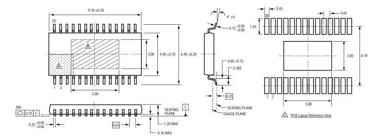
For reference only (reference JEDEC MO-153 AET) Dimensions in millimeters
