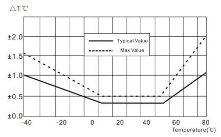
Figure 3. Typical and maximum temperature errors
