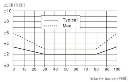
Figure 2. Typical and maximum humidity errors
