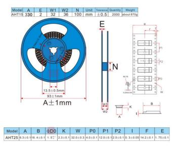
Figure 14. Packing tape and sensor location map
