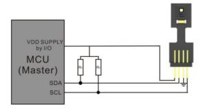
Figure 8. Typical application circuit
