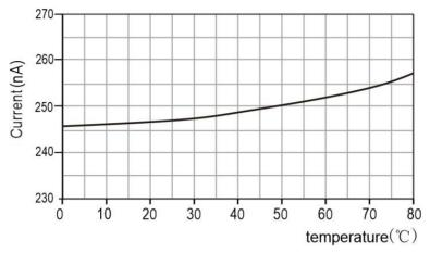
**Figure 6.** Typical supply current vs. temperature curve (sleep mode) when VDD=3.3V Please note: There is a deviation of approximately ±25% between these data and the displayed value.
