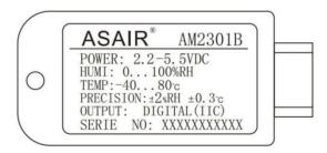
Figure 13. Sensor laser identification.
