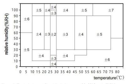
Figure 5. The typical error of humidity in the range of 0~80°C, unit: (%RH)
