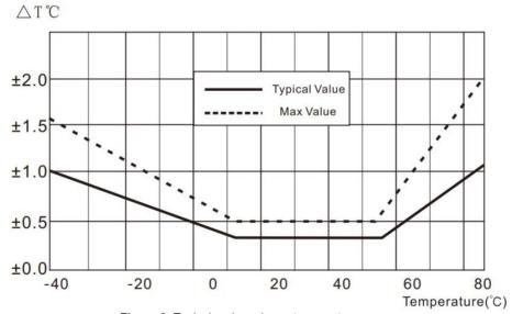
Figure 3. Typical and maximum temperature errors
