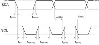
Figure 9. Timing diagram of digital input / output
