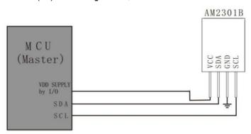
Figure 8. Typical application circuit
