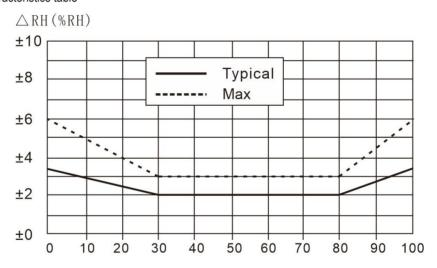
Figure 2. Typical and maximum humidity errors
