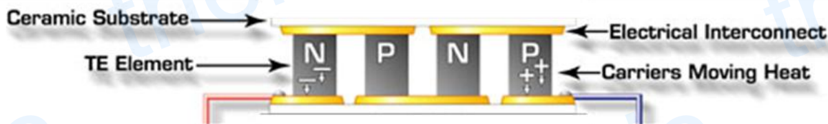
Figure 1 The structure of the Peltier modules
