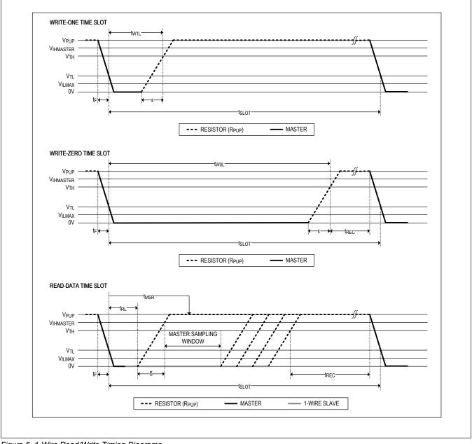
Figure 6. 1-Wire Read/Write Timing Diagrams
