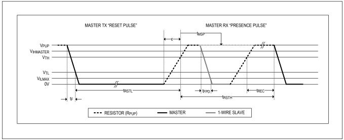
Figure 5. 1-Wire Reset/Presence-Detect Cycle
