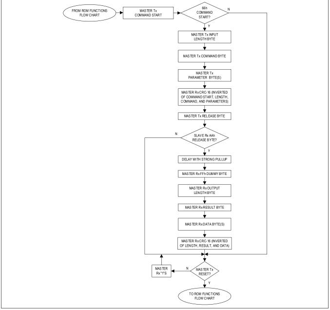
Figure 8. Device Function Flow Chart
