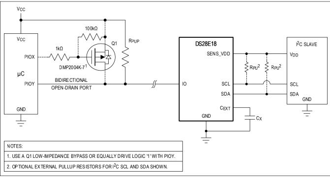
Figure 13. DS28E18 Configured as an I<sup>2</sup>C Master
