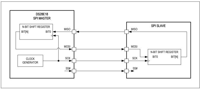
Figure 11. SPI Single Slave Network
