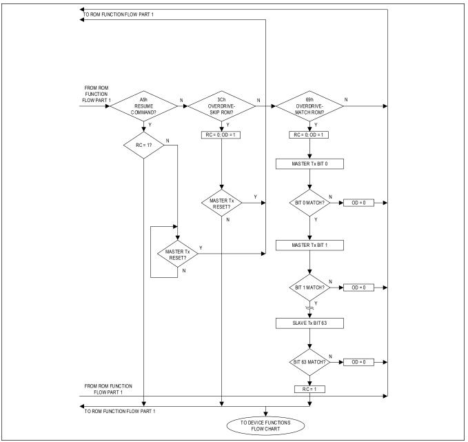
Figure 4. 1-Wire ROM Function Flow Part 2
