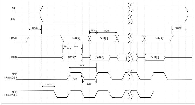
Figure 12. SPI Timing Diagram
