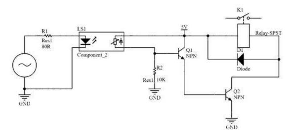
When the input current changes, the output current follows a linear change, driving the current of the two-stage transistor amplification circuit to change. When it reaches a certain value, the relay starts.
