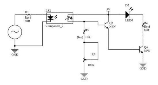
When the input current changes, the output current follows a linear change, driving the current of the two-stage transistor amplification circuit. The LED brightness driven by the transistor changes linearly. Adjusting the 100k adjustable resistor can change the driving LED current.
