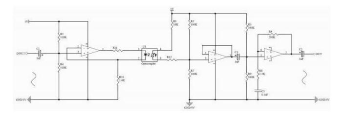
In audio systems, coupling between input voltage or current circuits to another level typically requires isolation. Optocoupler isolation has the characteristics of unidirectional signal transmission, complete electrical isolation between input and output, no impact on input at the output end, anti-interference, stable operation, and long contactless service life. Due to its superior linear output, this product has better performance in audio systems and can replace Cd output type optocouplers.
