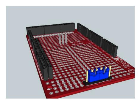
If you use the 6-pin male header jumpers to power the BUS, then you can only have +5V.
