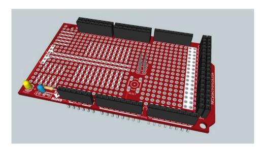
The RESET switch is necessary if you want to reset the chipKIT Max32 board from the top
