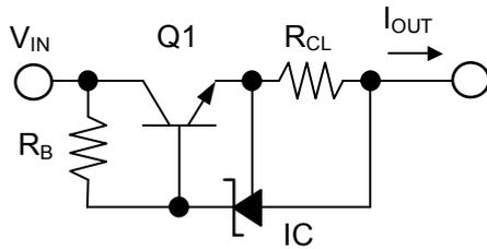
$$I_{OUT} = \frac{V_{REF}}{R_{CL}} + I_{KA}$$
