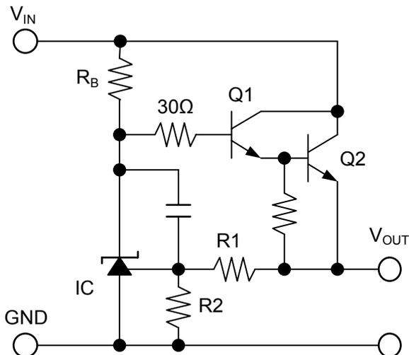
$$V_{OUT} = \left( \frac{R1}{R2} + 1 \right) \times V_{REF} + I_{REF} \times R1$$
