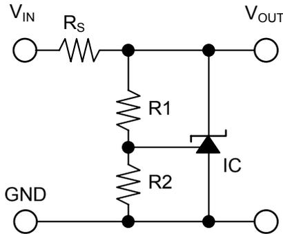
$$V_{OUT} = \left( \frac{R_1}{R_2} + 1 \right) \times V_{REF} + I_{REF} \times R_1$$
