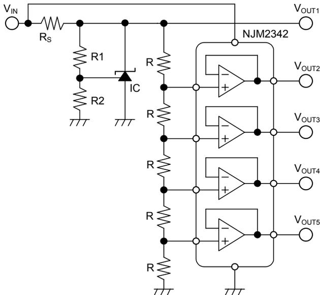
$$V_{OUT1} = \left( \frac{R1}{R2} + 1 \right) \times V_{REF} + I_{REF} \times R1$$
