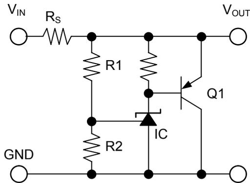
$$V_{OUT} = \left( \frac{R1}{R2} + 1 \right) \times V_{REF} + I_{REF} \times R1$$
