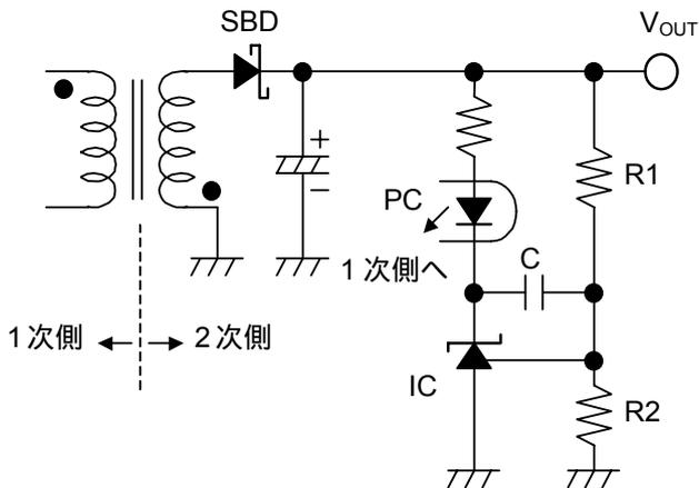
$$V_{OUT1} = \left( \frac{R1}{R2} + 1 \right) \times V_{REF} + I_{REF} \times R1$$
