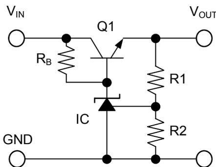
$$V_{OUT} = \left( \frac{R1}{R2} + 1 \right) \times V_{REF} + I_{REF} \times R1$$
