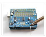
Solder each one of the pins into the shield to make a secure connection
