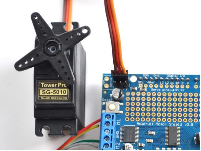
Hobby servos are the easiest way to get going with motor control. They have a 3-pin 0.1" female header connection with +5V, ground and signal inputs. The motor shield simply brings out the PWM output lines from Arduino pins 9 and 10 to two 3-pin headers so that its easy to plug in and go. They can take a lot of power so a 9V battery wont last more than a few minutes!
