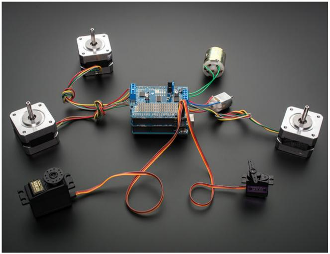
One of the cool things about this shield design is that it is possible to stack shields. Every shield you stack can control another 2 steppers or 4 DC motors (or a mix of the two)
