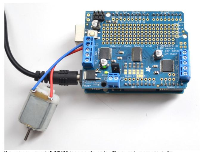
You must also supply 5-12VDC to power the motor. There are two ways to do this
