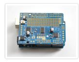
Place the assembled shield on top of the header-ed Arduino so that all of the short parts of the header are sticking through the outer set of pads
