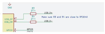
The RP2040 provides two pins to be used for Full Speed (FS) or Low Speed (LS) USB, either as a Host or Device, depending
