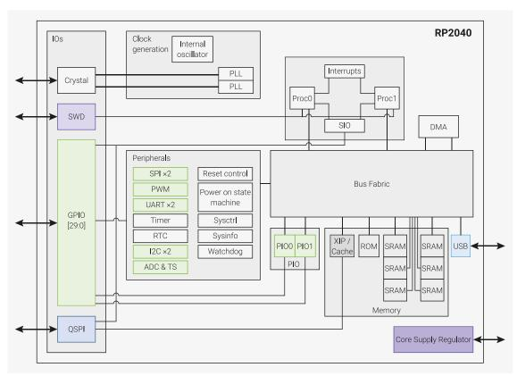
Code may be executed directly from external memory, through a dedicated SPI, DSPI or QSPI interface. A small cache improves performance for typical applications.
