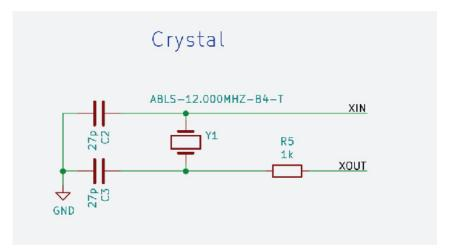
Strictly speaking, RP2040 does not actually require an external clock source, as it has its own internal oscillator. However, as the frequency of this internal oscillator is not well defined or controlled, varying from chip to chip, as well as with different supply voltages and temperatures, it is recommended to use a stable external frequency source. Applications which rely on exact frequencies are not possible without an external frequency source, USB being a prime example.
