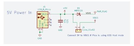
The **VSYS pin** is the main system power supply on Raspberry Pi Pico. From this supply, Raspberry Pi Pico generates its own 3.3V supply which is used to power RP2040, and also the 3V3 output pin of Raspberry Pi Pico which we can use to power circuits on our design.
