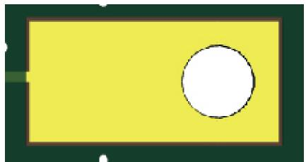
Each pin on Raspberry Pi Pico has two soldering options. You can either solder 0.1" headers using the through-holes, or alternatively, as Raspberry Pi Pico has castellated edges, where the pin extends to the edge of the board, and then down the edge of the PCB itself, it can be soldered down directly to a PCB.
