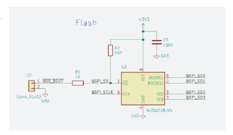
In order to be able to store program code which RP2040 can boot and run from, we need to use a flash memory, specifically, a quad SPI flash memory. The device chosen here is an W25Q128JVS device (**U2** in the Figure 7), which is a 128Mbit chip (16Mbyte). This is the largest memory size that RP2040 can support. If your particular application doesn't need as much storage, then a smaller, cheaper memory could be used instead.
