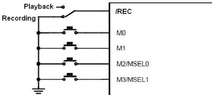
The memory will be divided to 4 messages averagely when both MSEL0 and MSEL1 pin float after chip reset
