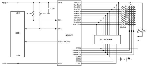
Note: 1. If RA0 and RA1 are Open, the I<sup>2</sup>C slave address (A0~A1) is set to low and A2 is always set to low.
