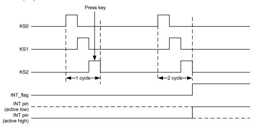
• Key pressed during a keyscan cycle period. (i.e. the key is pressed on the KS2 row)
