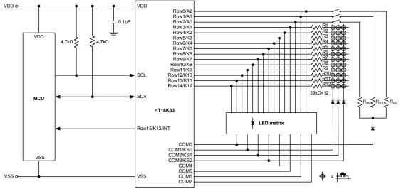
Note: 1. If  $R_{A0}$ ,  $R_{A1}$  and  $R_{A2}$  are Open, the I<sup>2</sup>C slave address (A0~A2) is set to low.
