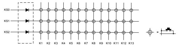
In this configuration, pressing three or more times may cause the OFF switches to be determined as being ON.
