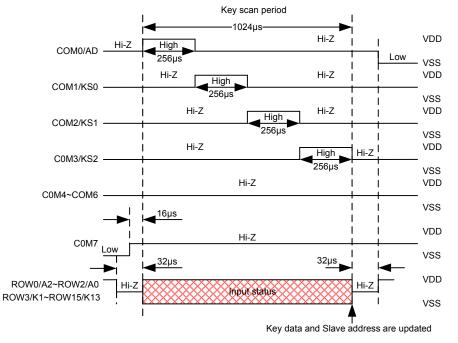
Note: The ROW/IN combined pin is set to a Row driver output.
