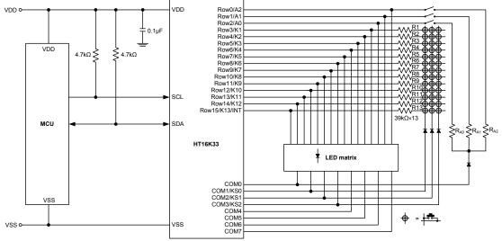
Note: 1. If  $R_{A0},\,R_{A1}$  and  $R_{A2}$  are Open, the  $I^2C$  slave address (A0~A2) is set to low.
