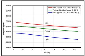
FIGURE 36-29: LFINTOSC Frequency, PIC16LF18313/18323 Only
