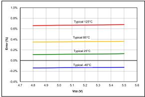
FIGURE 36-96: FVR Voltage Error (4x), PIC16F18313/18323 Only
