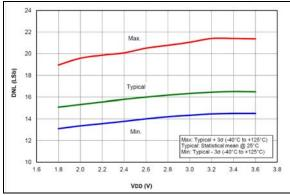
**FIGURE 36-73:** DAC INL Error, VDD = 3.0V, PIC16LF18313/18323 Only
