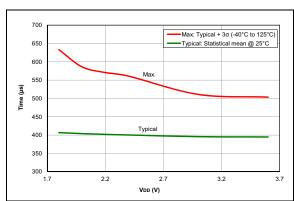
FIGURE 36-114: Wake From Sleep, LFINTOSC, PIC16LF18313/18323 Only
