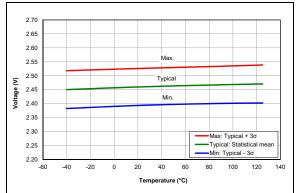
FIGURE 36-43: Brown-out Reset Voltage, Trip Point, (BORV = 1), PIC16F18313/18323 Only
