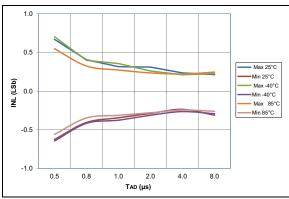
FIGURE 36-56: ADC 10-Bit Mode, Single-Ended INL, VDD = 3.0V, VREF = 3.0V, All devices
