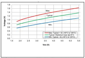
FIGURE 36-99: TTL Trip Thresholds, All devices
