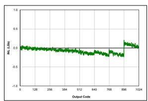
FIGURE 36-54: ADC 10-Bit Mode, Single-Ended INL, VDD = 3.0V, VREF = 3.0V, TAD = 8 µs, 25°C, All devices
