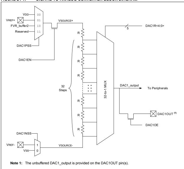
FIGURE 24-2: VOLTAGE REFERENCE OUTPUT BUFFER EXAMPLE
