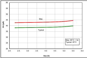
FIGURE 36-17: IPD, Fixed Voltage Reference (FVR), PIC16F18313/18323 Only
