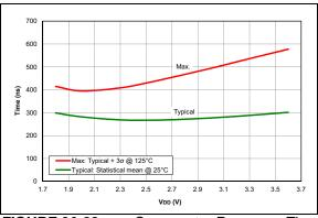
FIGURE 36-88: Comparator Response Time Rising edge, PIC16LF18313/18323 Only
