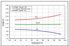
FIGURE 36-45: LPBOR Reset Voltage, PIC16LF18313/18323 Only
