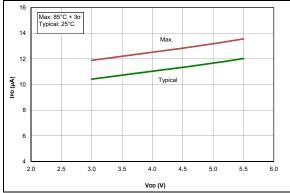
**FIGURE 36-19:** IPD, Brown-out Reset (BOR), BORV = 1, PIC16F18313/18323 Only
