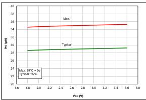
**FIGURE 36-22:** IPD, Comparator, PIC16LF18313/18323 Only
