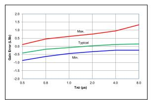
FIGURE 36-65: ADC 10-Bit Mode, Single-Ended Gain Error, VDD = 3.0V, VREF = 3.0V, -40°C to 85°C, All devices
