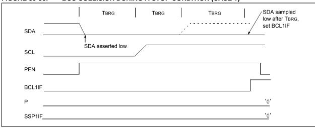
FIGURE 30-39: BUS COLLISION DURING A STOP CONDITION (CASE 2)
