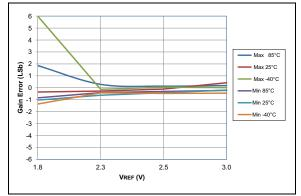
FIGURE 36-59: ADC 10-Bit Mode, Single-Ended Gain Error, VDD = 3.0V, TAD = 1 μs, All devices
