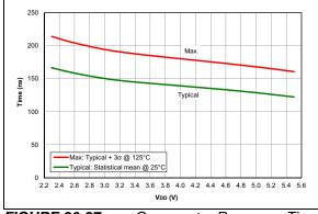
FIGURE 36-87: Comparator Response Time Falling edge, PIC16F18313/18323 Only
