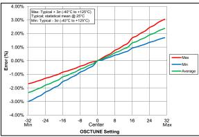
FIGURE 36-104: OSCTUNE Center Frequency, PIC16LF18313/18323 Only
