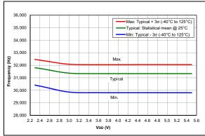
FIGURE 36-30: LFINTOSC Frequency, PIC16F18313/18323 Only
