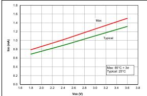
FIGURE 36-7: IDD, HFINTOSC Mode, Fosc = 16 MHz, PIC16LF18313/18323 Only
