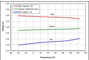
FIGURE 36-105: POR Release Voltage, All devices
