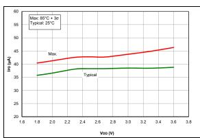
FIGURE 36-16: IPD, Fixed Voltage Reference (FVR), PIC16LF18313/18323 Only
