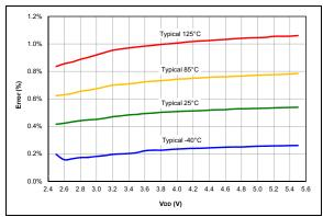
**FIGURE 36-93:** FVR Voltage Error (1x), PIC16F18313/18323 Only
