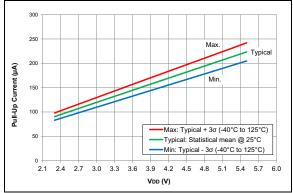
**FIGURE 36-31:** Weak Pull-Up Current, PIC16F18313/18323 Only
