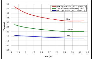
FIGURE 36-67: ADC RC Oscillator period, PIC16LF18313/18323 Only
