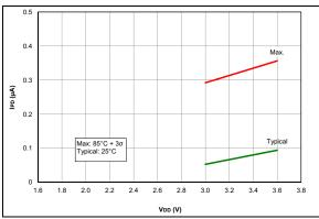
FIGURE 36-20: IPD, Low-Power Brown-out Reset (LPBOR = 0), PIC16LF18313/18323 Only
