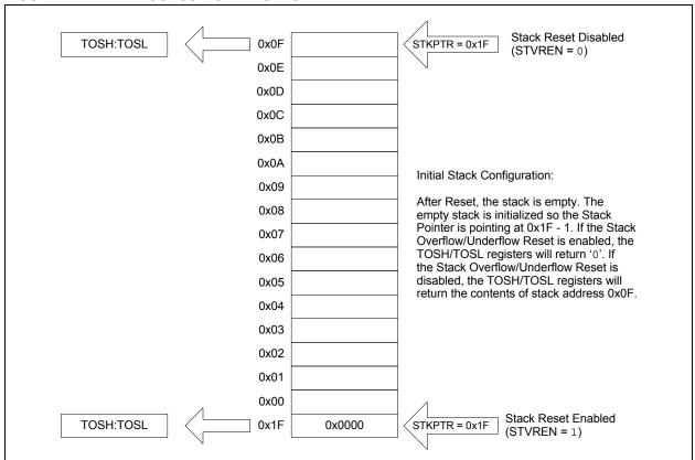
FIGURE 4-5: ACCESSING THE STACK EXAMPLE 2
