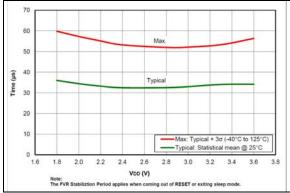
**FIGURE 36-91:** FVR Stabilization Period, PIC16LF18313/18323 Only
