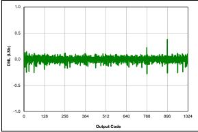
FIGURE 36-49: ADC 10-Bit Mode, Single-Ended DNL, VDD = 3.0V, VREF = 3.0V, TAD = 1 µs, 25°C, All devices
