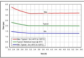
FIGURE 36-68: ADC RC Oscillator period, PIC16F18313/18323 Only
