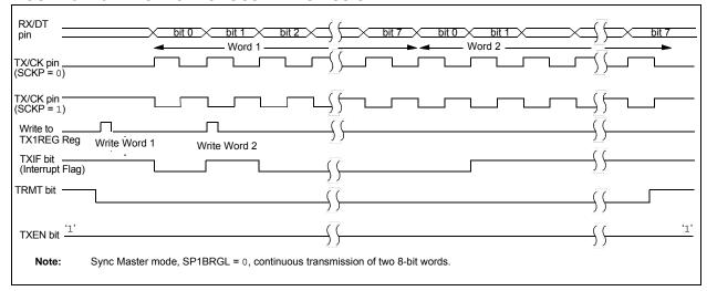
FIGURE 31-11: SYNCHRONOUS TRANSMISSION (THROUGH TXEN)
