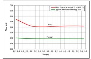
FIGURE 36-113: Wake From Sleep, VREGPM = 1, LFINTOSC, PIC16F18313/18323 Only
