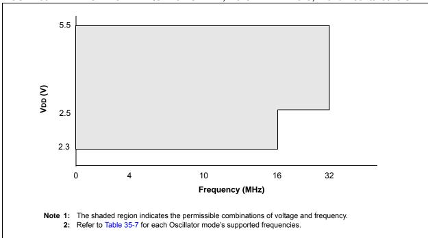
FIGURE 35-2: VOLTAGE FREQUENCY GRAPH, -40°C ≤TA ≤+125°C, PIC16LF18313/18323 ONLY
