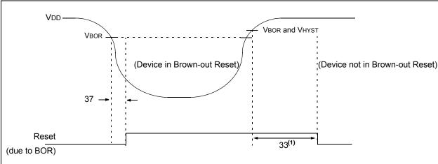
**Note 1:** 64 ms delay only if  $\overline{\text{PWRTE}}$  bit in the Configuration Word register is programmed to '0'. 2 ms delay if  $\overline{\text{PWRTE}} = 0$ .
