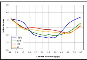
FIGURE 36-81: Comparator Hysteresis, Normal Power Mode (CxSP = 1), VDD = 5.5V, Typical Measured Values, PIC16F18313/18323 Only
