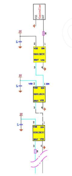
In the practical application circuit, the signal input and output pins of the IC signal input and output pins should be connected to the signal input and output terminals. In addition, in order to make the IC chip is more stable, even the capacitance between beads is essential back;
