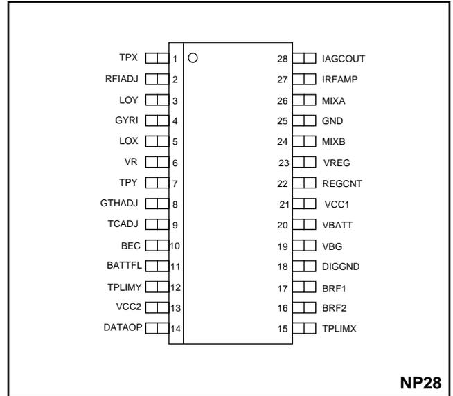
Fig.1 Pin connections
