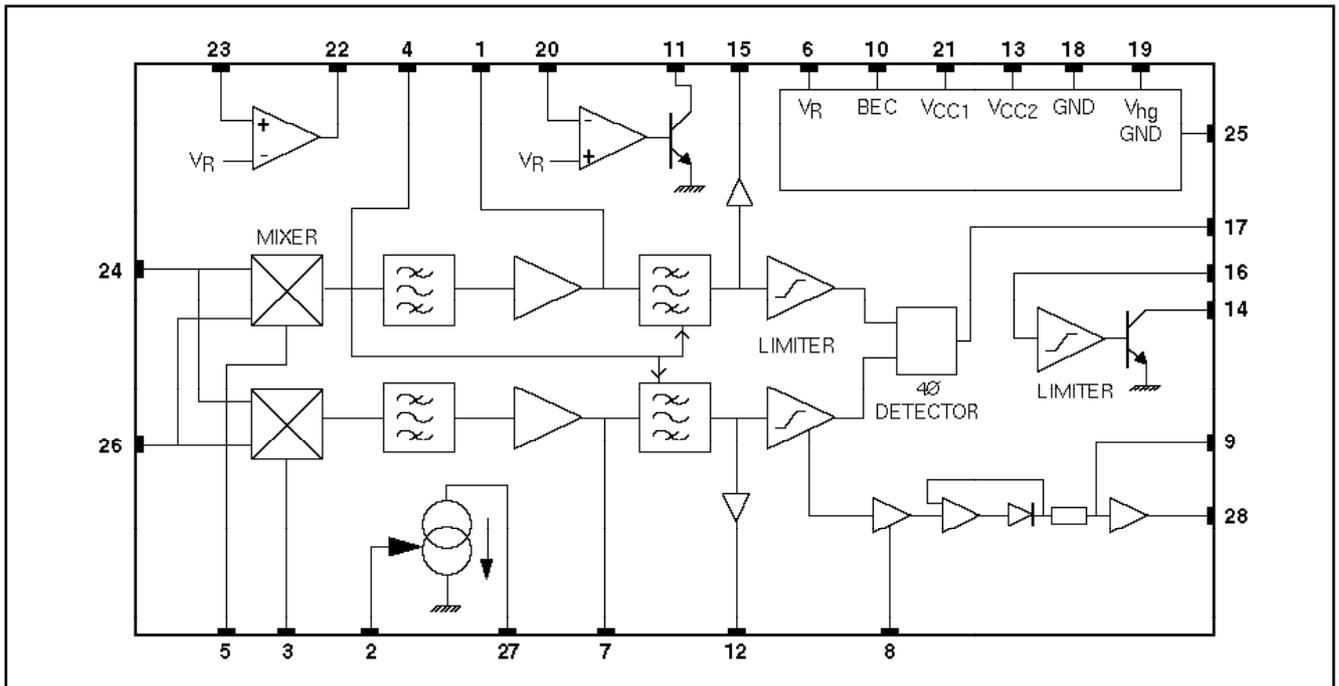
Fig.2 Block diagram of SL6609
